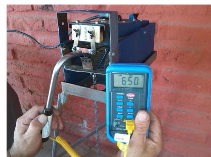
Pyrometer indicating proper blade temperature of 650°C.
